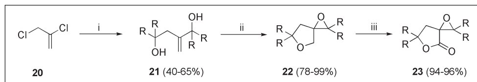
Fig. 4. Reagents: (i) Li, C_{10}H_8 (2.5%), R^1R^2CO = Et_2CO, (CH_2)_4CO, (CH_2)_5CO, O(CH_2CH_2)_2CO, adamantan-2-one, THF, -78 to 0^\circ C ; (ii) R^3R^4C(O)CHR^5 = MeCH(O)CH_2, PhCH(O)CH_2, n-C_6H_{13}CH(O)CH_2, Et_2C(O)CH_2, PhMeC(O)CH_2, (n-C_5H_{11})_2C(O)CH_2, cyclopentene oxide, cyclohexene oxide, methylenecyclohexane oxide, methyleneadamantane oxide, 0^\circ C , then H_2O ; (iii) I_2, Ag_2O, THF ; (iv) BH_3 \cdot THF , then H_2O_2 \cdot NaOH ; (v) PCC or Ru(PPh_3)_3Cl_2, CH_2Cl_2 .
